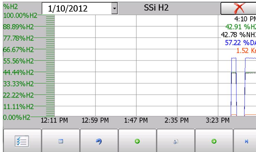
The Chart Display shows between 1 hour and 24 hours of process variable data on the screen and can be scrolled back to view all of the data stored on the hard drive. The vertical timelines change as the time changes on the screen.
