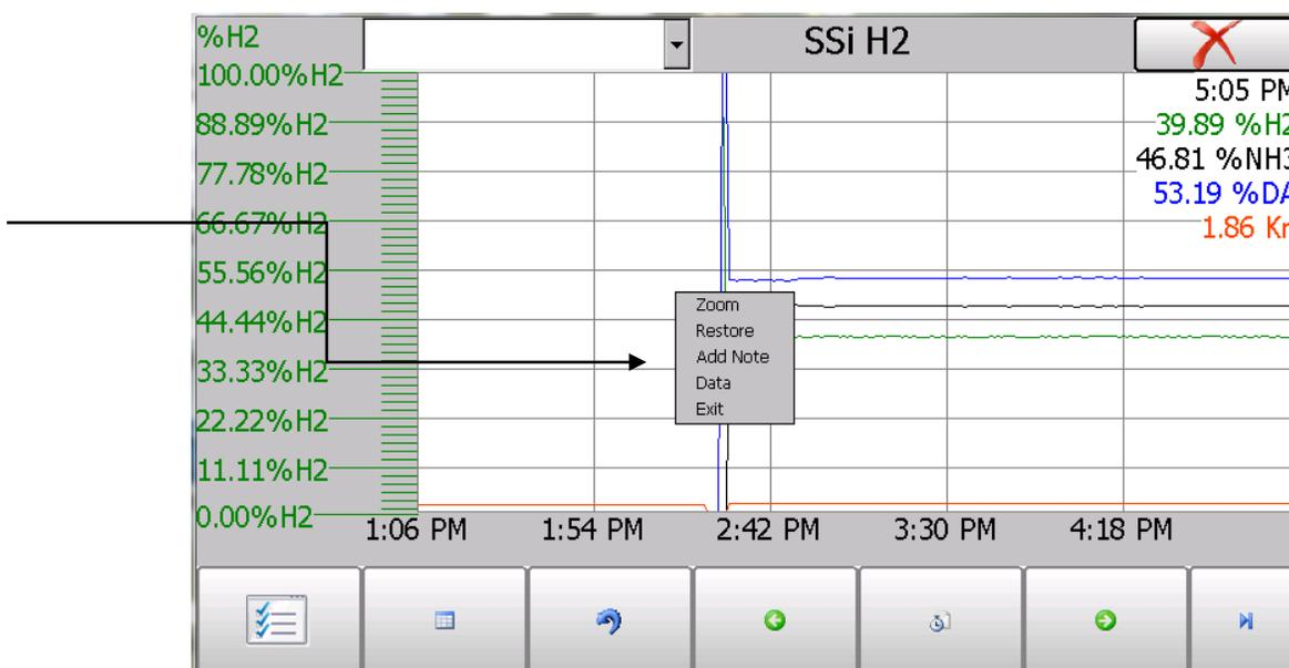
The **Zoom** option will allow the user to zoom in on a particular part of the screen. Once this has been selected, the user can take a stylus or a finger and create a box around the desired data. Once the user releases the stylus or finger, a zoom is no longer possible, and the user will need to re-select the option from the sub-menu to zoom in again.
