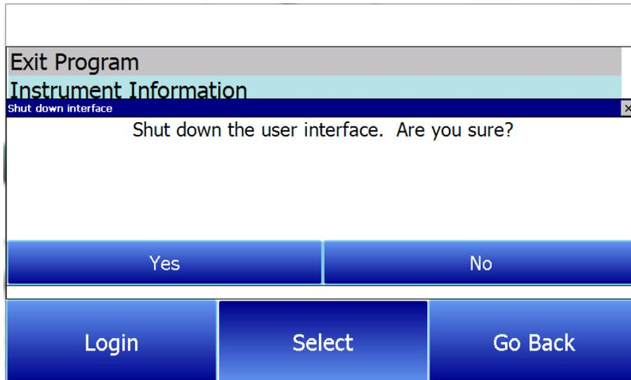
Once the PH<sub>2</sub> interface is shut down, you will see the operating system screen. The following procedure is typical for changing the IP address.
