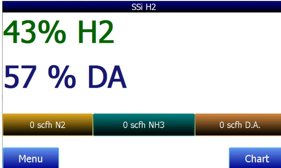
The home screen also displays the flow of N<sub>2</sub>, NH<sub>3</sub>, and D.A. These values can be entered by the operator when the instrument is in the mode to evaluate Kn or %DA. This is discussed further under the Instrument Configuration section. The **Menu** button in the bottom left-hand corner will take the operator to the configurable options within the controller. The **Chart** button in the bottom right-hand corner of the screen will display the data trend chart.
