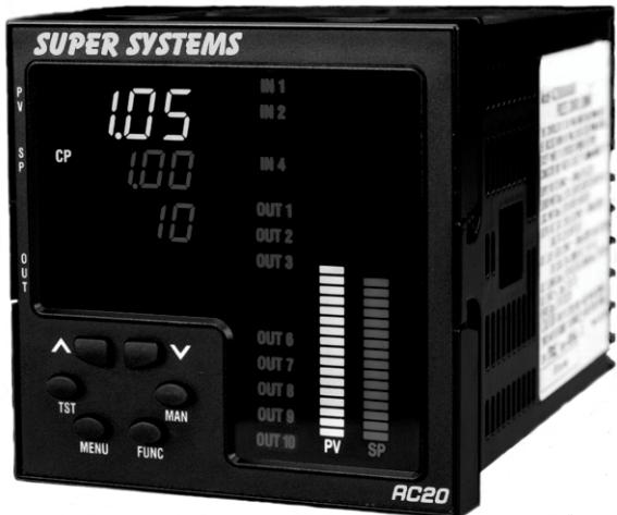
The **AC20** controller is designed to control both endothermic generators and atmosphere furnaces. To accomplish both, the **AC20** can display and control on three units of measure: % Carbon, Dew Point or probe millivolts. In addition, Probe resistance, probe temperature, COF, H<sub>2</sub>F and probe recovery can be displayed.
