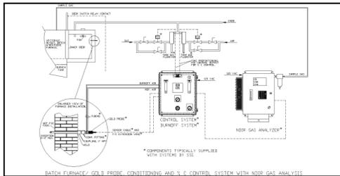
Atmosphere composition, independent of the probe reading, can be monitored and used to improve the accuracy of the carbon calculation using the probe only input. This is performed by adjusting the correction factor (COF/PF) configured in the atmosphere control instrumentation. The adjustment process is implemented using a dedicated, continuous gas monitoring system focusing on three gases that are the largest components of the furnace atmosphere.
