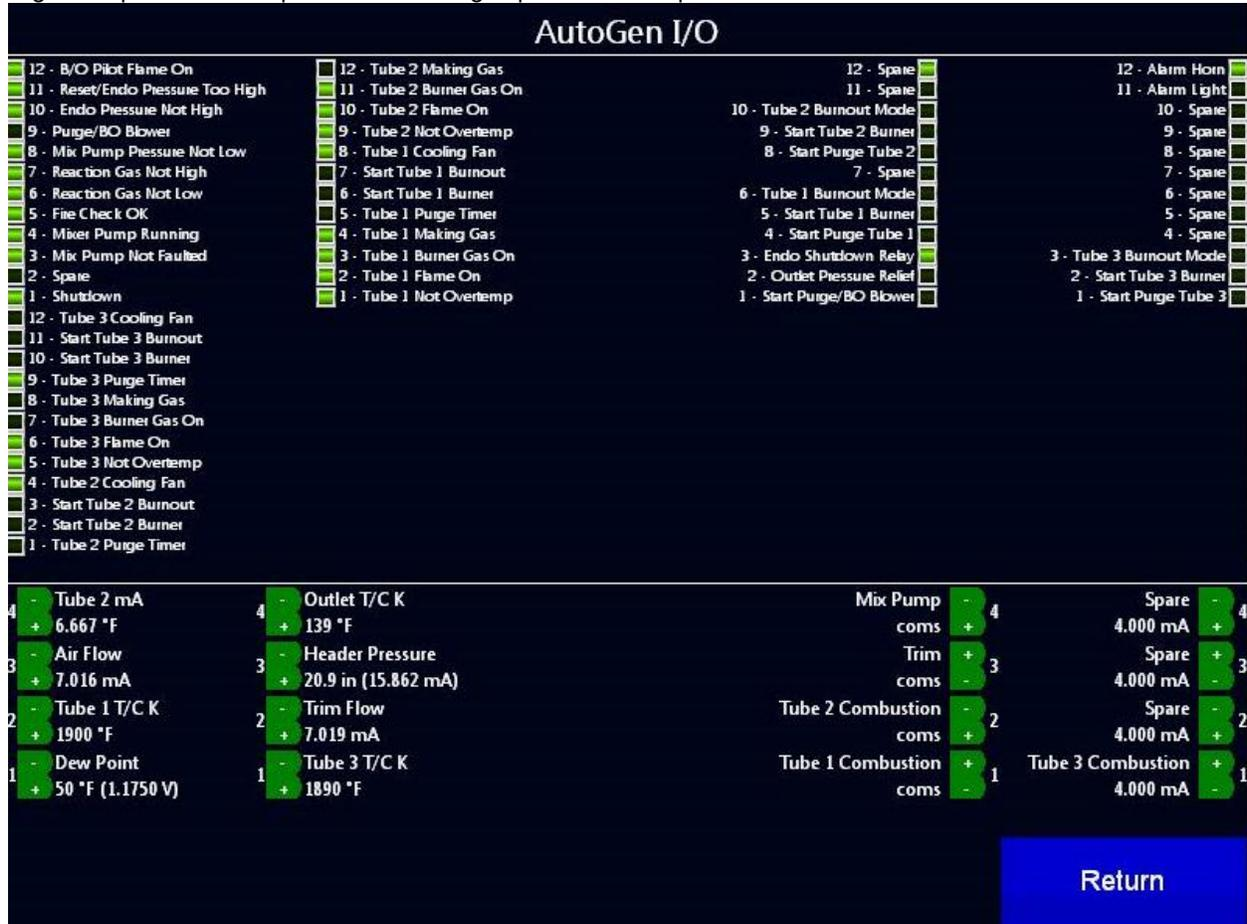
Analog I/O is shown on the bottom of the screen (below the horizontal line). Digital I/O is shown on the top (above the line). Inputs are shown on the left side of the screen, and outputs are shown on the right side. See the Digital I/O menu and Appendix 4 for more information on these options.
