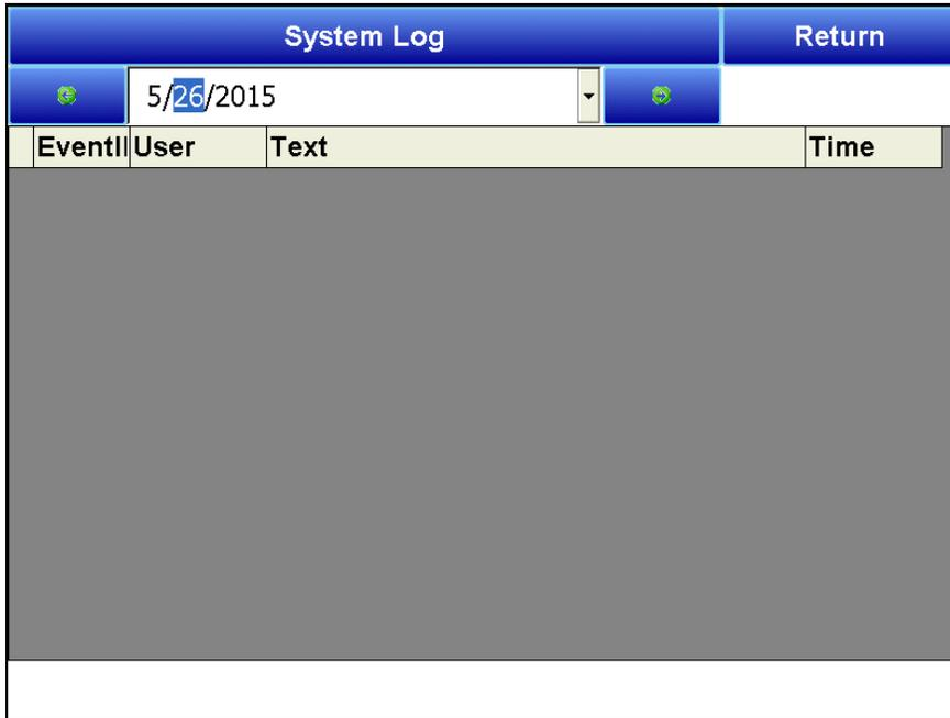
Clicking on the button that displays the log type (**System Log**, **Alarm Log**, or **Cycle Log**) will allow the user to select the type of log file to view.
