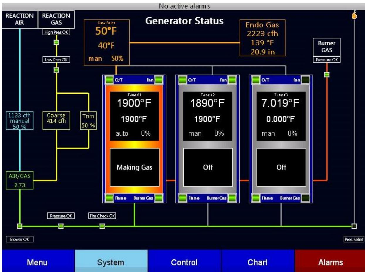
The generator tubes are represented in the large rectangular boxes near the center of the screen. Current temperature, setpoint, control mode, and output percentage are shown in these
