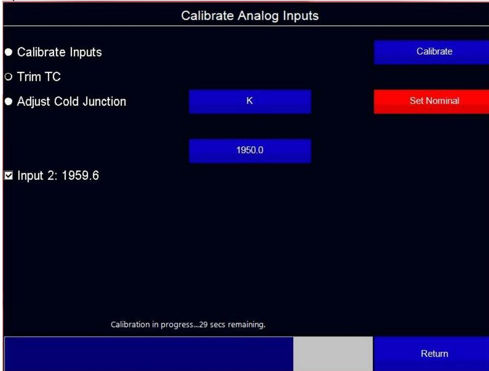
Adjust Cold Junction allows the user to directly adjust the temperature of the cold junction at the terminals where the TC connects to the AutoGen.
