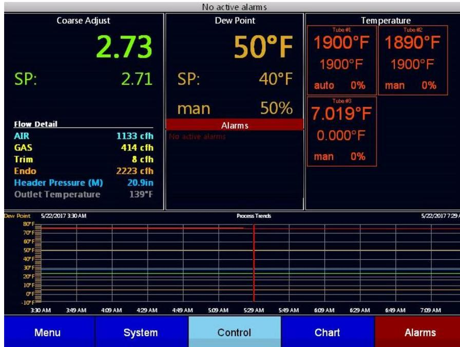
Parameters related to coarse adjustment, dewpoint, and temperature are shown in separate panes along the top of the screen. Parameters related to flow are shown in the leftmost pane. Current alarms are shown in the middle pane (near the center of the screen) and are also
