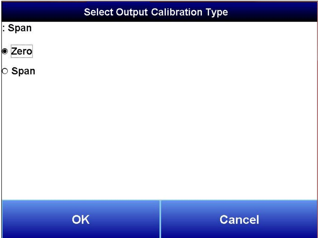
3. Tap Prep for calibration. This causes the analog output to generate the minimum or maximum output (4 or 20 mA).
