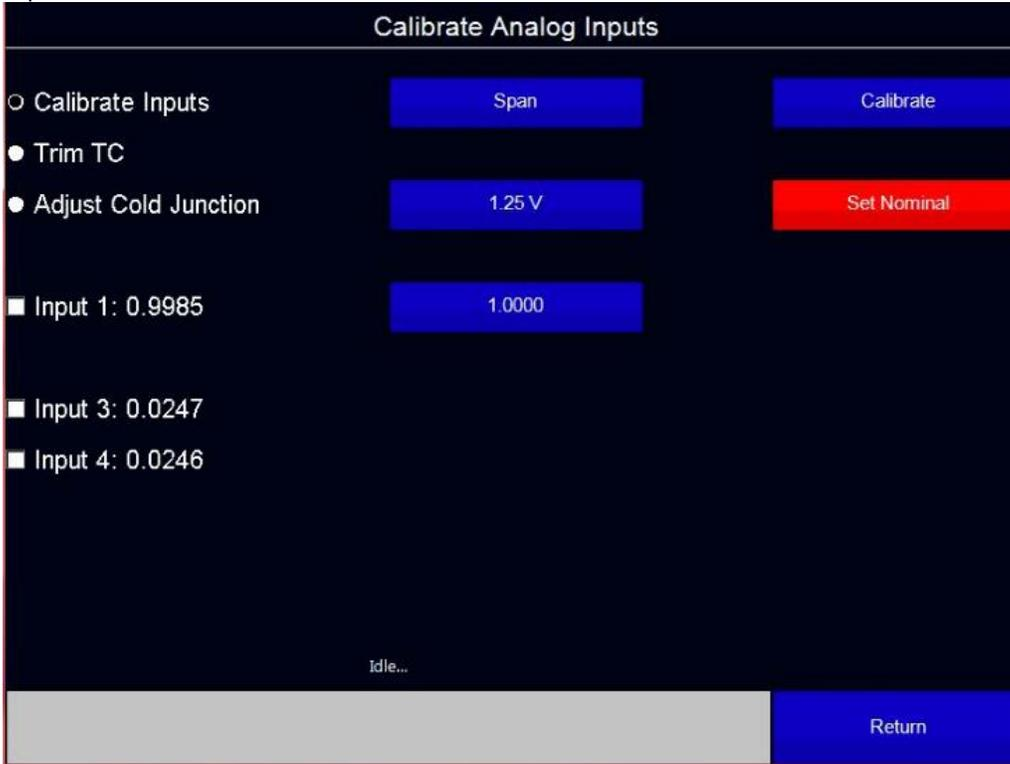
4. If Span calibration is selected an additional button will be below the range button. This is the suggested signal for the selected range. This value can be edited; however, this is not recommended.
