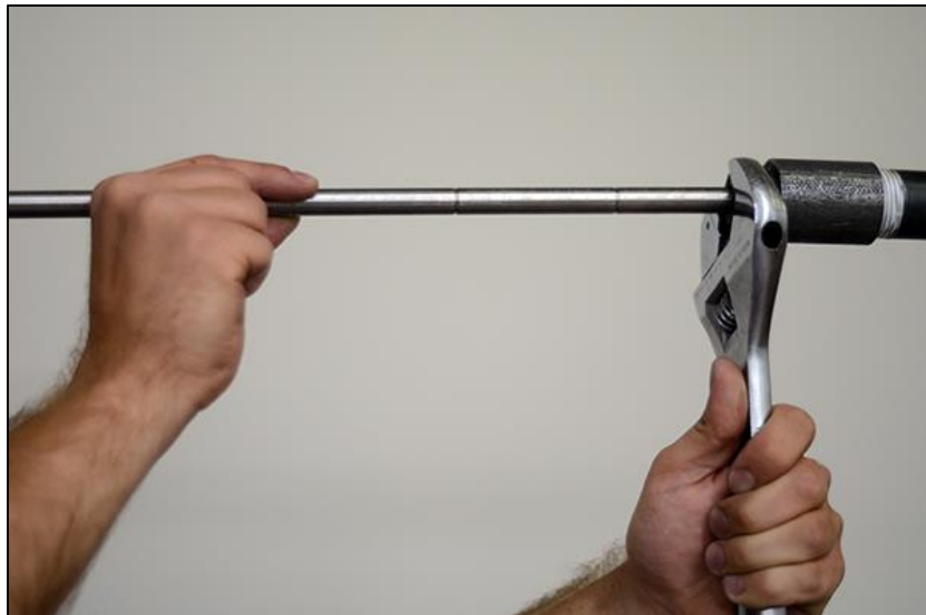
Figure 11 - Tightening port connector with wrench
