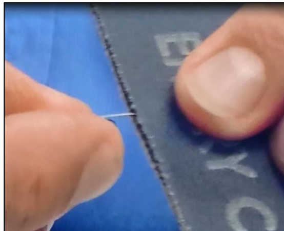
Figure 13 - Using emery cloth on wire coil
