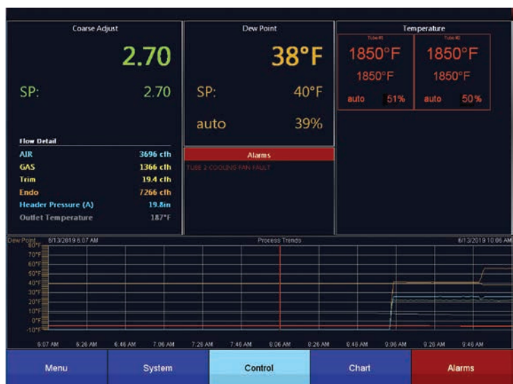
Fig. 2. Automatic adjustment the ratio of air to gas
