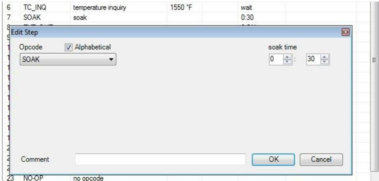
Under the Soak Time in the upper left hand corner, there are two numeric entry boxes. The left most numeric entry box is for time in hours. The right most numeric entry box is for time in minutes. To modify these times, either the Up or Down arrows can be pressed, or the desired time can be entered into the boxes from the keyboard. Once the correct time has been entered, press the OK button in the bottom right corner of the Edit Step box.
