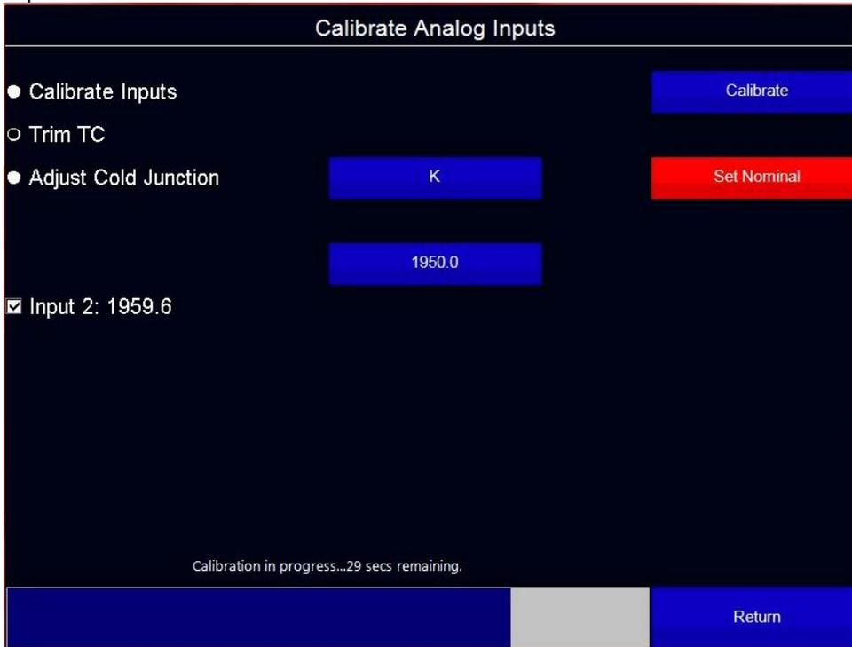
Adjust Cold Junction allows the user to directly adjust the temperature of the cold junction at the terminals where the TC connects to the controller.
