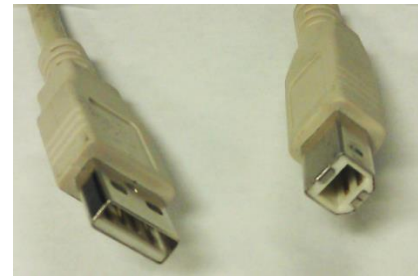
USB connection types Standard-A (left), Standard-B (right)
