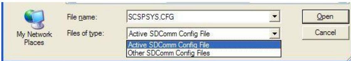
By selecting Files of type: Other SDComm Config files, you will be able to edit any files that have "scspsys" in the filename. Examples: scspsys.bak, scspsys\_old.cfg, scspsys\_save.txt etc.
