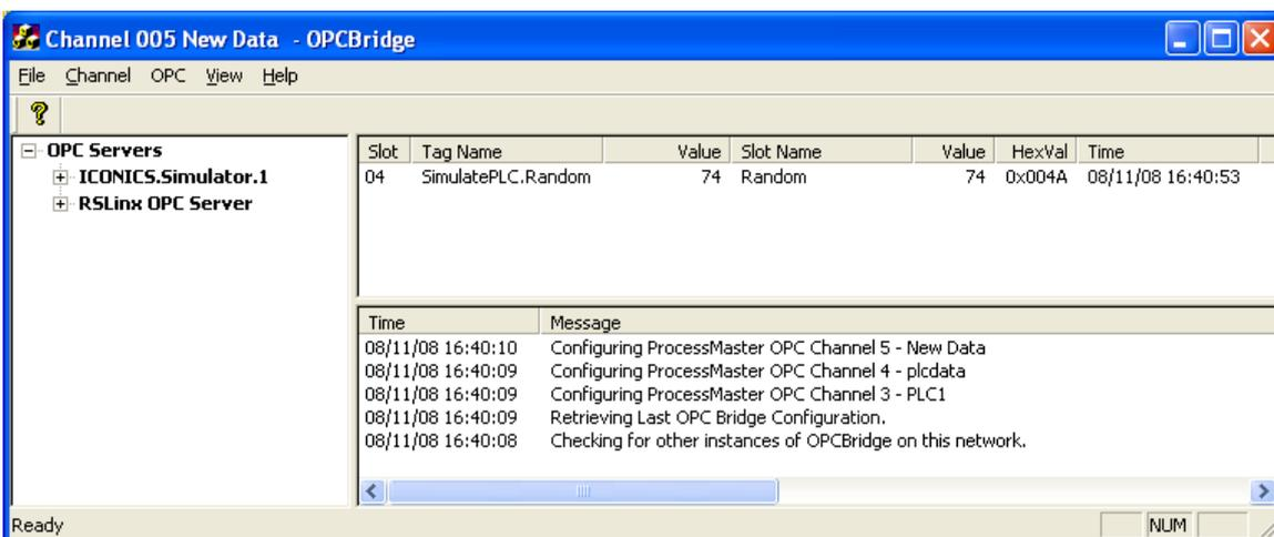
The configured slot data appears in the data window showing the slot number, the server tag name, the server value, the SuperData slot name, the SuperData slot value, the value in hex and the last update date and time.
