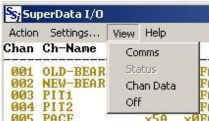
The View Menu is used to select the **Comms**, **Status** or **Chan Data** view. This menu may also be used to turn the view **off**. When the view is turned off, the display will stop updating until the comm. or Status view is selected. The **Comms view** displays messages and errors for selected channels as configured in settings.
