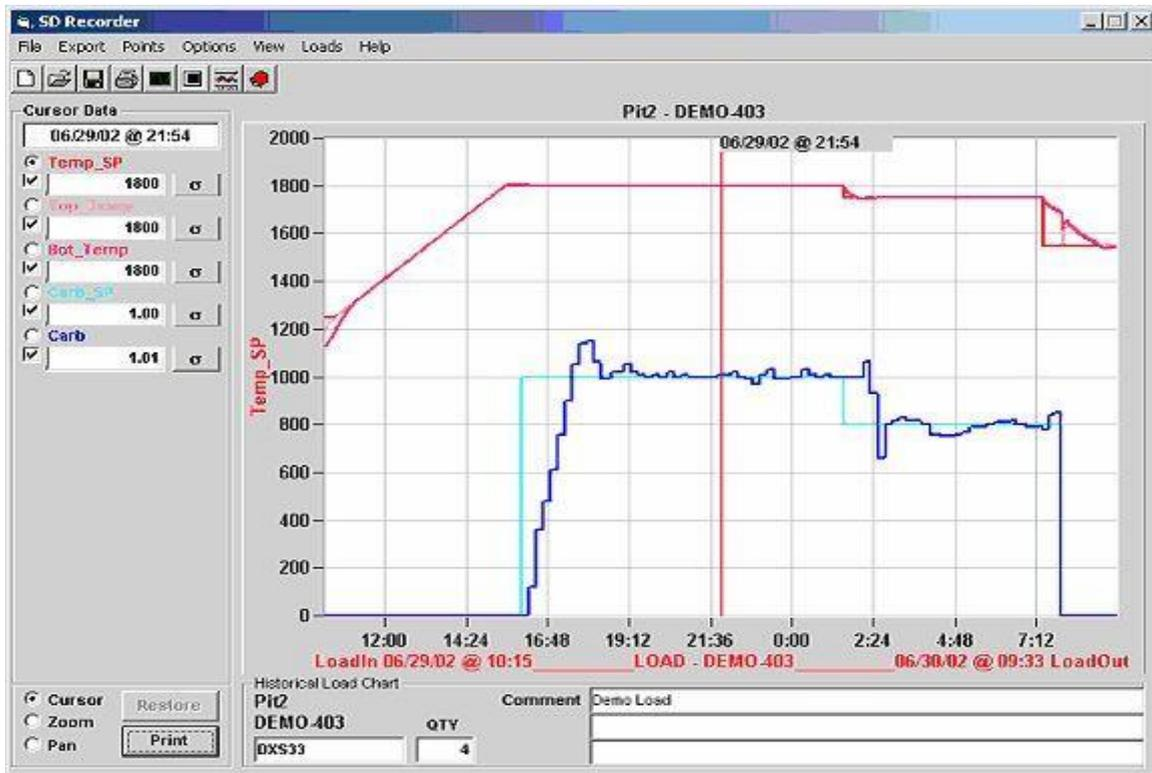
Historical Load Charts are displayed differently from a normal chart. The Horizontal Time scale is fixed by the "Load In" and "Load Out" times and there are no scroll buttons or window width selector. The Loads Database data is displayed below the chart. The database data (part, qty and comment fields) may be edited from here. When any of the data is edited, a save button will appear in the lower right corner. When printing, the database data will be printed with the chart.
