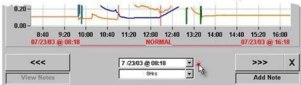
The chart opens with a default "window width" of 12 Hrs. In the "realtime" mode, the right scroll button and the "realtime" button are disabled (dimmed).
