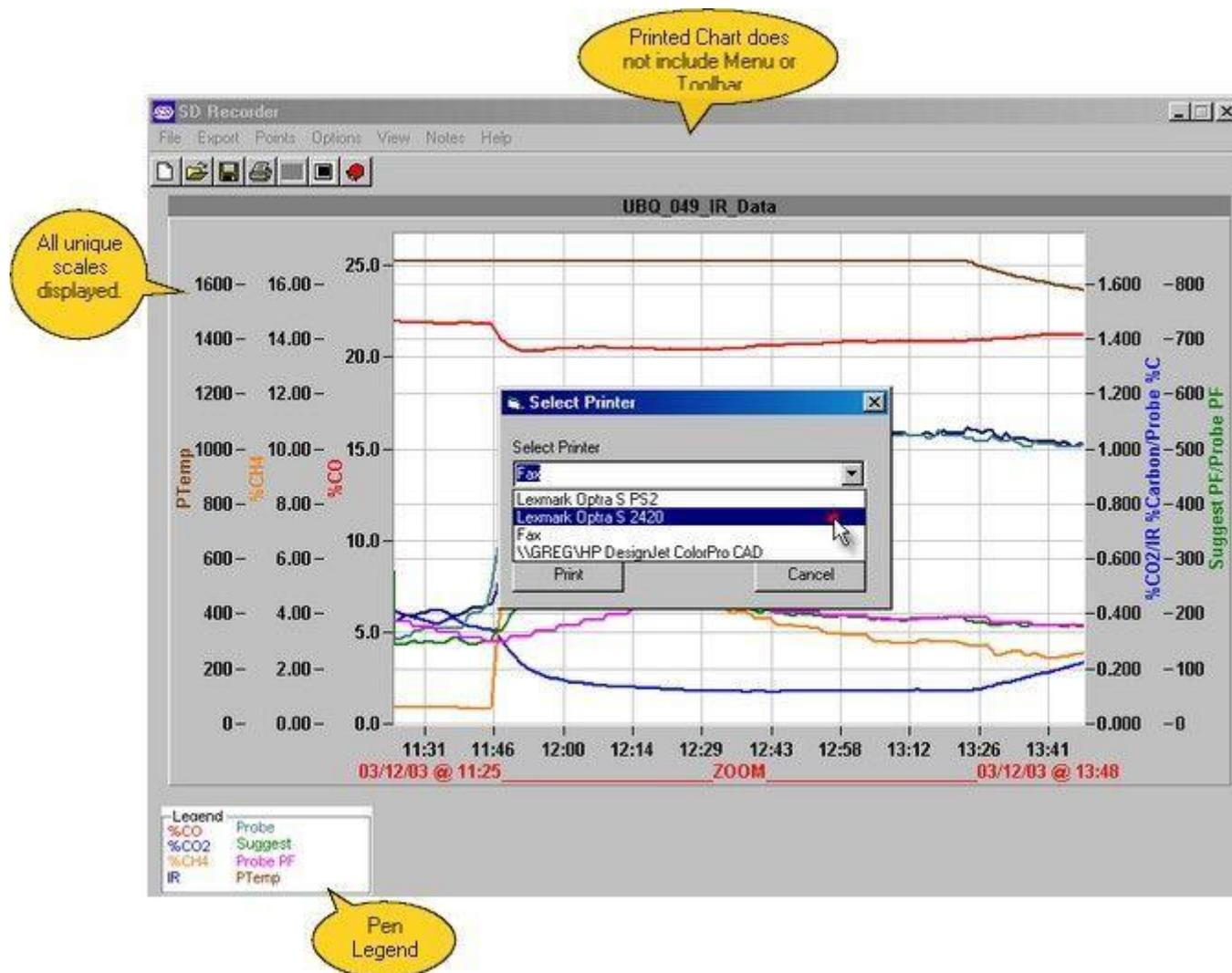
In this mode, the cursor, cursor data and chart controls are not displayed. A chart legend and all unique scales will be displayed. Select a Printer and click "Print" to send to the printer or "Cancel" to return without printing.
