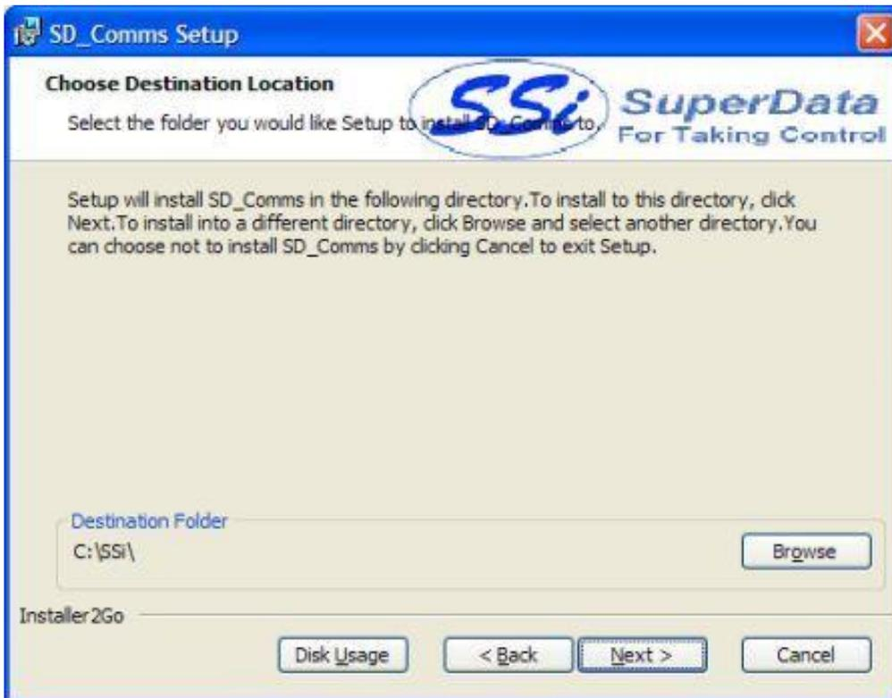
The next screen will prompt the user for the download location. The default location is "C:\SSi". Note: The installer will automatically create a "Bin" folder to install the files to. For example, if the default location, "C:\SSi\" is used, then the files will be installed to "C:\SSi\Bin".
