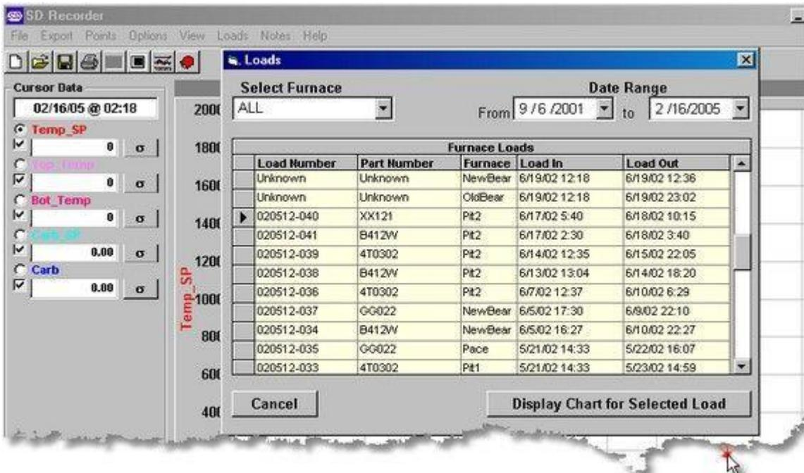
The **Loads** Menu is only available when SDRRecorder is configured to use a Load Tracking Database. Clicking on Loads opens a Load Selector Dialog. Selecting a Load from the Dialog and clicking "Display Chart for Selected Load" will open the chart for the selected Load. Note: The Loads Menu is not available when using the "AltData" option.
