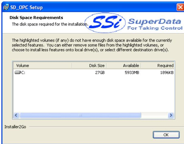
Clicking on the **Disk Usage** button will display the available computer drives onto which the application can be downloaded, as well as the total space, available space and total space required. Clicking on the **OK** button will close out the disk usage screen.
