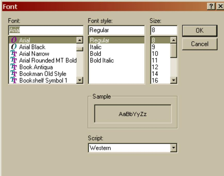
The Font selector is the common dialog for fonts. All available system fonts are listed; all possible styles and sizes for the selected font are selectable here, as well. Users should be careful of using very unusual fonts, as every computer must have the font on the system to use the selected font. Installing fonts is easy, but it is just one more detail. Among the most readable variable width fonts are MS Sans Serif and Arial. Courier is a good choice in fixed width fonts.
