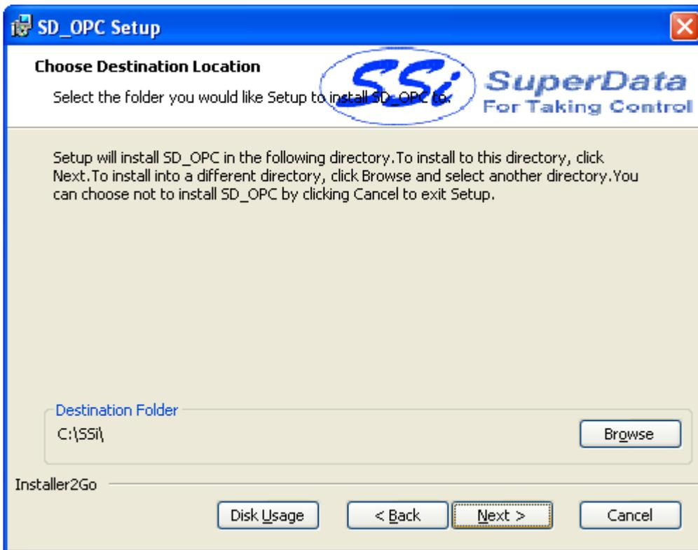
The screen will prompt the user for the download location. The default location is "C:\SSi\". Note: The installer will automatically create a "Bin" folder to install the files to. For example, if the default location, "C:\SSi\" is used, then the files will be installed to "C:\SSi\Bin".
