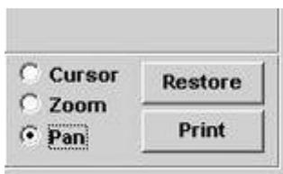
To pan the view, hold the left mouse button down and drag the mouse horizontally across the chart. The chart view window will follow the cursor. Use the restore button to undo the pan view.
