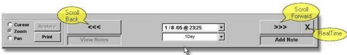
**Scroll Buttons** – The left and right scroll buttons scroll the chart view backwards or forwards by one half the display width. Using these buttons refreshes the data and will cancel any Zoom or Pan in effect.
