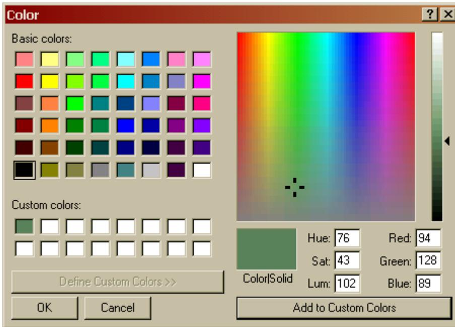
Add to Custom Colors will apply a new color to the Custom Color box selected on the left. Note: if a box is not selected on the left, the first Custom Color will be overwritten. This will not affect properties originally using the replaced color, as colors do not operate on indexes anymore.
