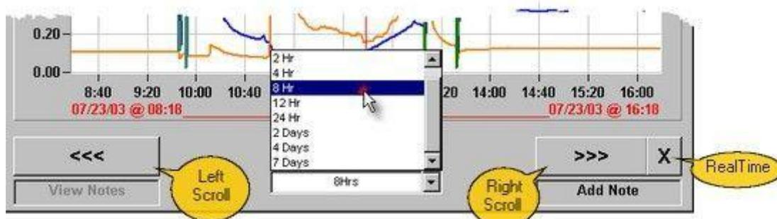
The window width may be changed from 1 Hour thru 7 days. Changing the window width will cause the data to be refreshed and the chart will be redrawn. The Left scroll button will cause the chart to exit realtime mode and move the chart back in time by ½ of the window width. The right scroll button will move the chart forward in time by ½ of the window width. You may resume "realtime" mode by clicking on the "realtime" button next to the right scroll button.
