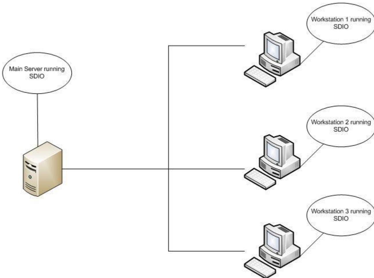
Remote channels may be mapped by "channel" OR by "channel/slot". When mapping by channel, all slots from the remote channel are mapped to corresponding slots in the local channel. This reduces configuration and has the advantage that Realtime screens and SDRrec charts can be the same on both computers with the possible exception of the channel number.
