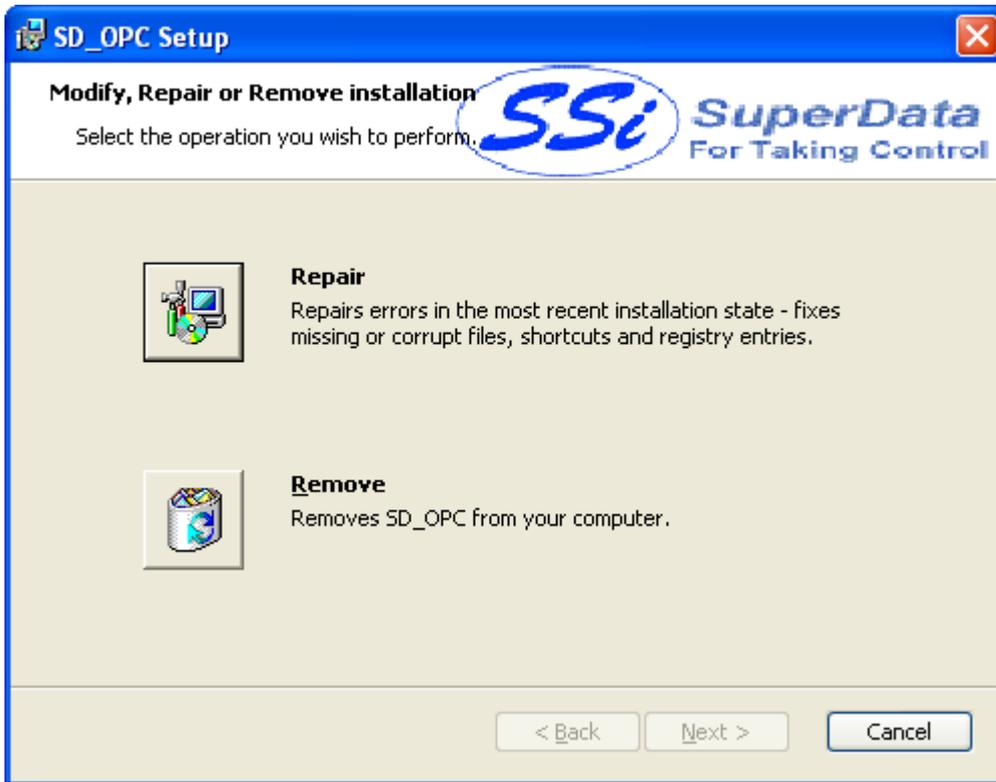
The installer will either re-install the software (**Repair** button) or remove the software from the computer (**Remove** button). Clicking on the **Cancel** button will cancel the actions. The user will have to confirm the cancellation. Note: the installer does not remove any subfolders in the main SSI folder. These files will have to be manually removed.
