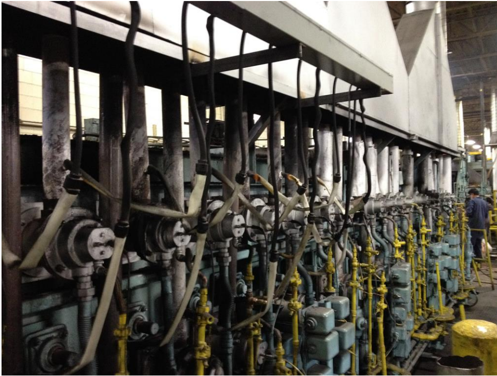
Typical Continuous Furnace Installation
