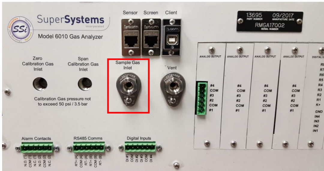
Sample Inlet Port Used for Sample Line Calibration
