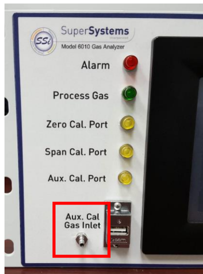
Gas Inlet Port for Auxiliary Calibration
