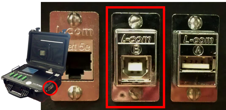
Figure 21 - Location of USB connection point for connecting data logger to local computer
