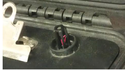
Figure 47 - Location of Ambient (External) Thermistor
