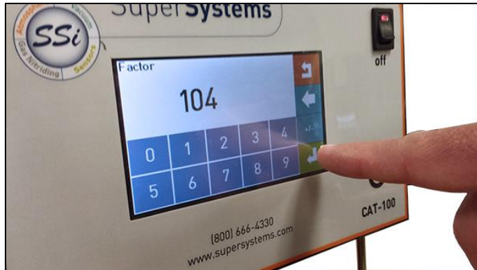
Figure 7 – Entering a new Coil Factor
