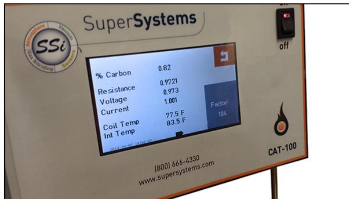
Figure 8 – Detail screen with new Coil Factor shown
