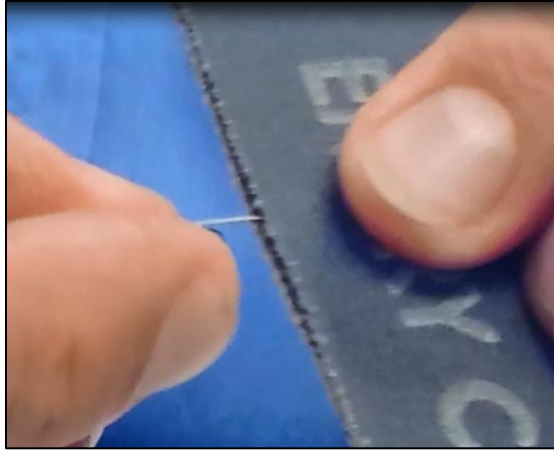
Figure 18 - Using emery cloth on wire coil
