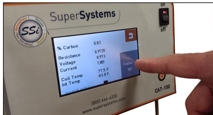
Figure 6 - Detail screen with Coil Factor box
