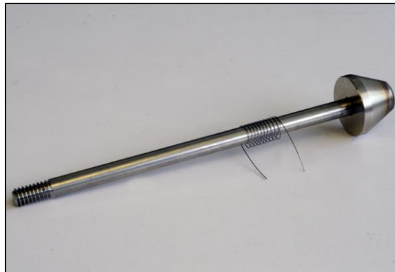
Figure 4 - Wire coil placed on rod screw
