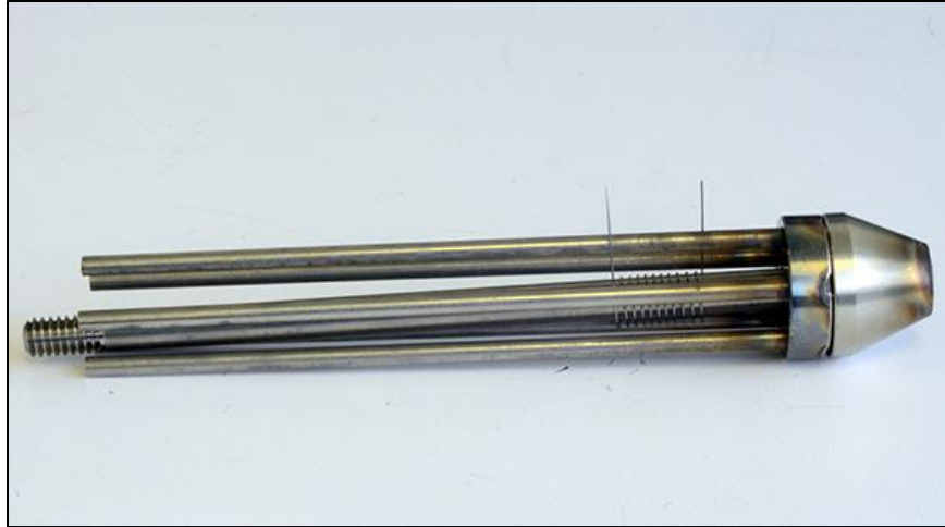
Figure 5 – Rod screw inserted through opening in protective cage
