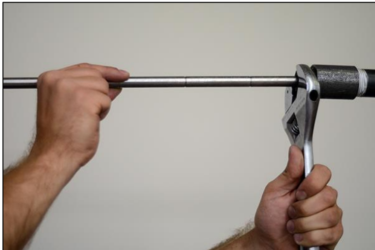
Figure 16 - Tightening port connector with wrench
