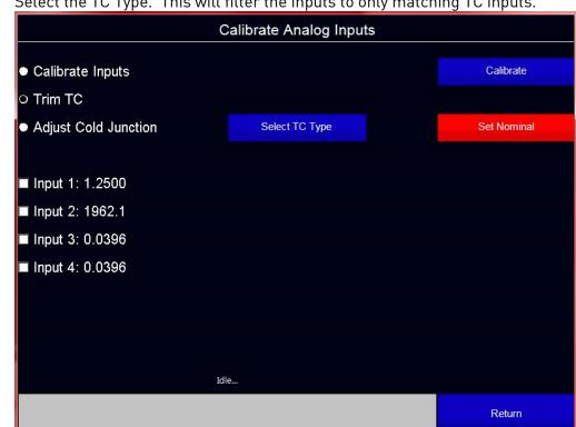
1. Select the TC Type. This will filter the inputs to only matching TC inputs.
