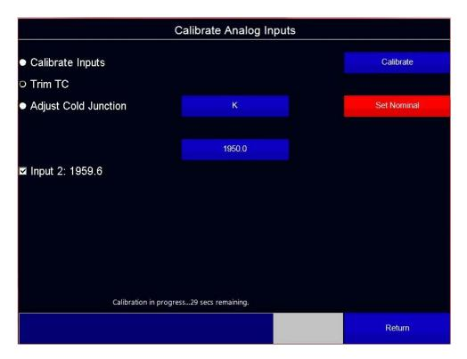
Adjust Cold Junction allows the user to directly adjust the temperature of the cold junction at the terminals where the TC connects to the controller.
