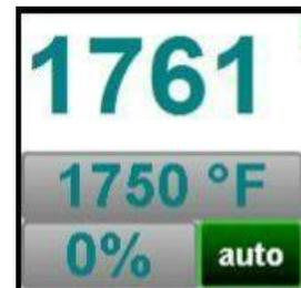
If the displayed value does not equal the value being sourced, then a Cold Junction Calibration may be necessary. To begin, note the difference between the displayed temperature and the sourced temperature. This is the adjustment that will be made in the "Cold Junction" menu. For example:
