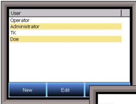
If the "Advanced" option is selected, then clicking on the **Users** button will allow the user to create or modify user information for the Touchscreen. *Note – Once the "Advanced" option is selected, a user name will need to be entered when logging into the menu system. A user name will need to be provided even if the Level 1 or Level 2 code is being used.*
