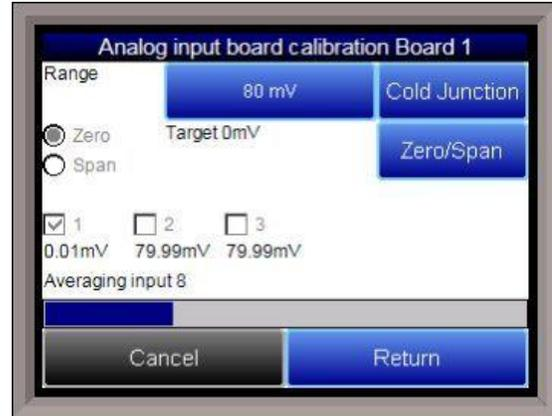
For a zero calibration, the recommended value to source is **0 mV**. The user can also individually select each input (one through three/five) to calibrate, where Check = yes (calibrate) and No Check = no (do not calibrate). Click on the **Calibrate** button to begin the calibration.
