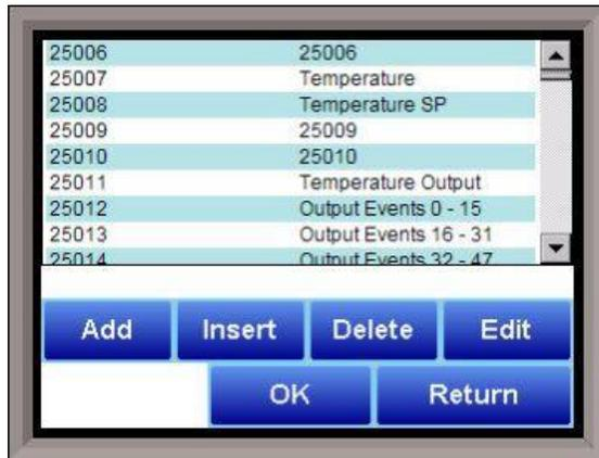
To add a new description, click on the **Add** button. To insert a new description, click on the **Insert** button. To delete a description, click on the **Delete** button. To edit an existing description, click on the **Edit** button. The Add or Insert feature will only create valid descriptions if there are existing data values without descriptions. Click on the
