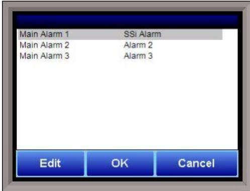
This menu option will allow the user to configure the text for the three main alarms on the 9130. Highlight the alarm to be changed and click on the **Edit** button. This action will display the on-screen keyboard, which will allow the user to modify the alarm text. To save the changes to the alarm text, click on the **OK** button. Clicking on the **Cancel** button will not save any of the changes made.
