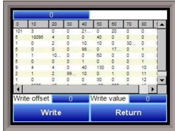
The number box in the top left of the screen is the beginning register to read from. This will default to 0 when the screen starts. To read registers 100 – 199, edit the value to read "100". *Note – changing the value will automatically begin the read process. This process could take a few seconds to complete.*
