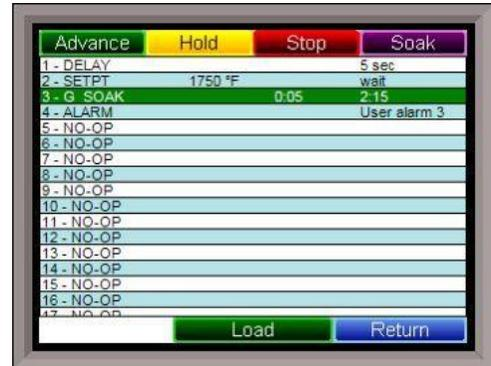
The recipe screen has a total of seven buttons that will allow the user to load up a recipe, as well as control the recipe and acknowledge an alarm.
