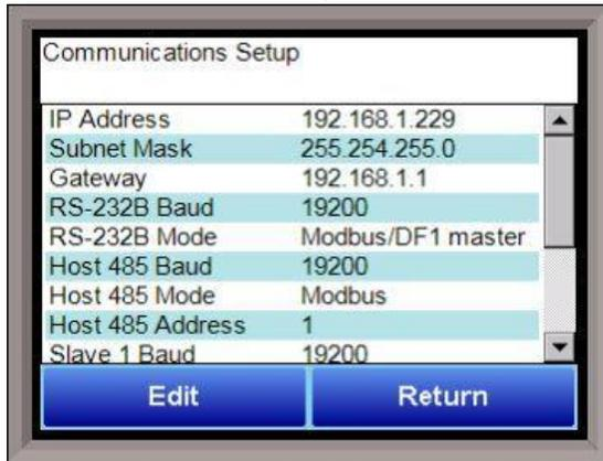
**Warning:** Changes to this screen should not be made without consulting SSi at 513-772-0060. This screen will show the Ethernet and RS-232/RS-485 communications information for the 9130 controller.
