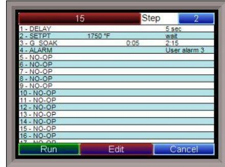
While reviewing the program that is about to be run, each step can be modified. Highlight a
