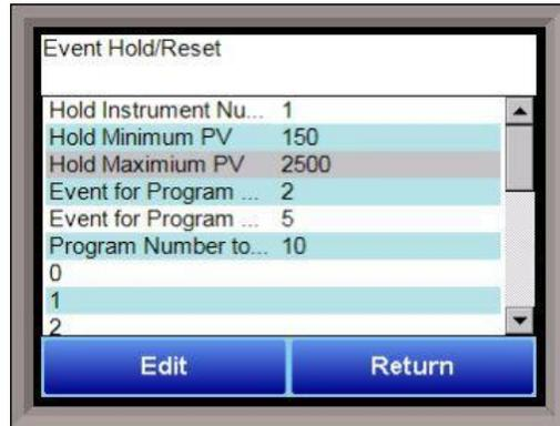
The Event Hold/Reset menu option provides the user manual control of actual event outputs. This is useful when testing wiring and field devices.
