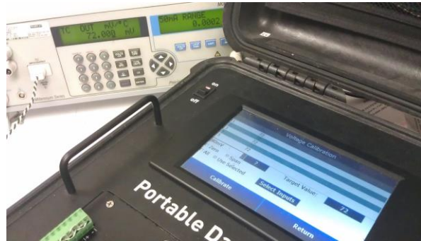
Figure 41 - Voltage Calibration (Span) Ready to Begin
