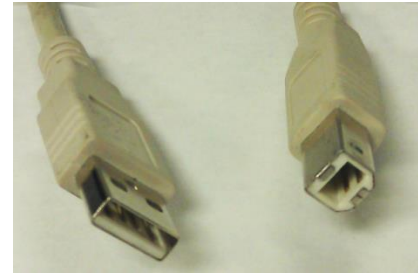
USB connection types Standard-A (left), Standard-B (right)
