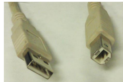
Figure 22 - USB connection types Standard-A (left), Standard-B (right)
