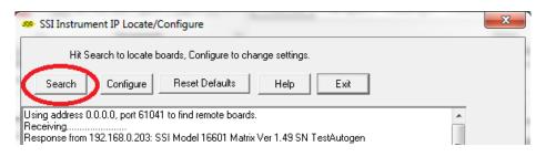
4. Look for identifying text in the list of instruments. It includes the type of instrument and serial number. It also provides the IP Address information for the sensor.
