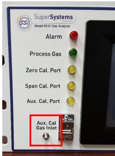
Gas Inlet Port for Auxiliary Calibration
