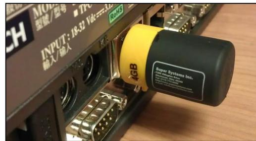
Figure 59 - Inserting USB Drive into USB Port on Touch Screen Device
