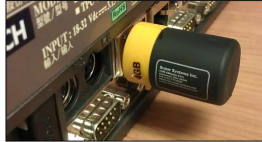
Figure 45 - Inserting USB Drive into USB Port on Touch Screen Device
