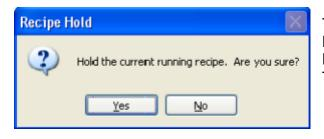
The **Hold** button will put the recipe on hold, but it will not stop the recipe. To hold a recipe, click on the **Hold** button. The user will have to confirm the action.
