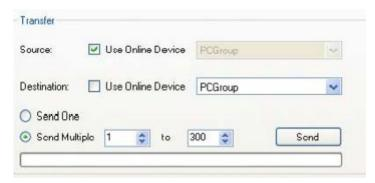
The Transfer section will allow the user to transfer one or more recipes from one location to another. The "Source" field could either be the currently connected device ("Use Online Device"), or one of the offline groups ("PCGroup"). The "Destination" field could either be the currently connected
