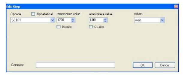
The drop-down list under "Opcode" allows the user to select the specific opcode that will be used in the recipe step. If a temperature value or an atmosphere value is needed, these can be set using the up or down arrows, or by just typing in the value. If these are not needed, check the "Disable" checkbox and the boxes will become unavailable.
