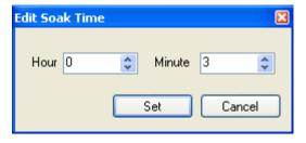
The current soak time will be displayed initially. To set a new soak time, change the hours and/or minutes to the desired values and click on the **Set** button. **Note — This change** will only last for the current soak and will not be a permanent change. To cancel the change, click on the **Cancel** button.
