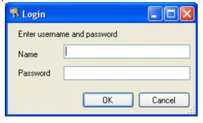
To login as Supervisor, enter "Supervisor" as the user name and enter the level 1 pass code as the password. The user name is not case-sensitive. If the login is successful, the login button will show (gold).
