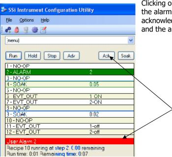
Clicking on the **Ack** button will acknowledge the alarm. Once the alarm has been acknowledged, the **Ack** button will disappear, and the alarm text will disappear as well.
