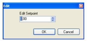
Click on the atmosphere set point box (middle box in the left column) to alter the set point. Enter the new value or use the up and down arrows to select the new value. Click on the **OK** button to set the new atmosphere set point. Clicking on the **Cancel** button will cancel the action.
