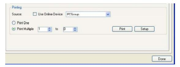
The Printing section allows the user the ability to print out recipes. The "Source" field could either be the currently connected device ("Use Online Device"), or one of the offline groups ("PCGroup").
