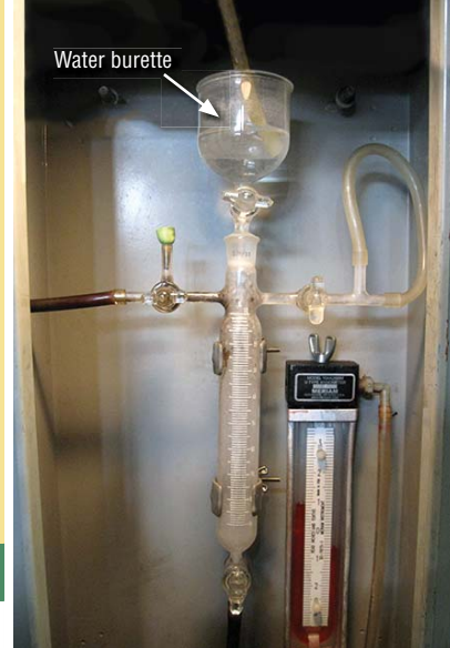
Fig. 2. Use of water burette in testing %DA
