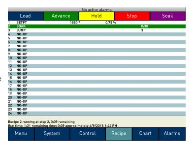
The recipe screen has a total of five buttons that will allow the user to load up a recipe, as well as control the recipe and acknowledge an alarm.
