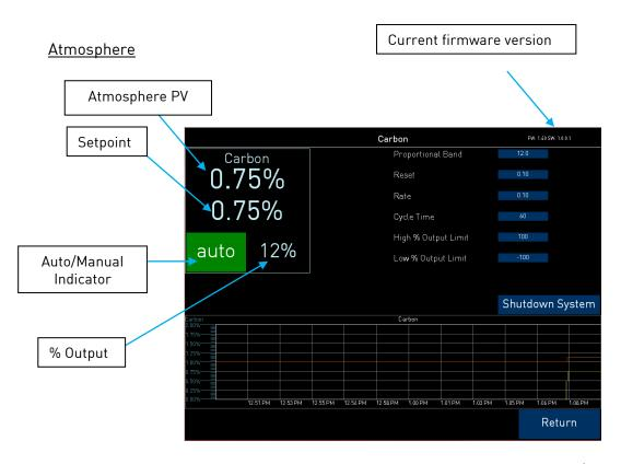
The Atmosphere screen displays the current temperature PV, the current SP, Auto/Manual mode indicator, and % output.
