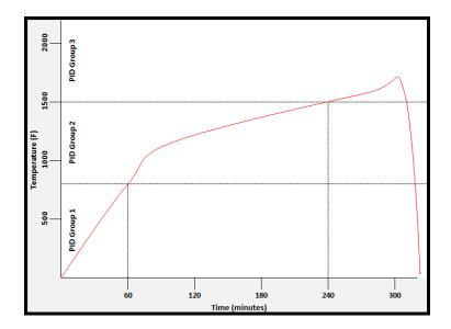
In the example above, proper use of the Tuning Assistant allows the user to find the following optimal PID settings for the following temperature ranges:
