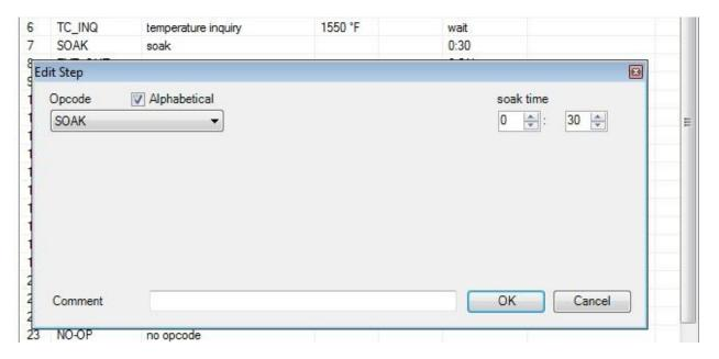
Under the Soak Time in the upper left hand corner, there are two numeric entry boxes. The left most numeric entry box is for time in hours. The right most numeric entry box is for time in minutes. To modify these times, either the Up or Down arrows can be pressed, or the desired time can be entered into the boxes from the keyboard. Once the correct time has been entered, press the OK button in the bottom right corner of the Edit Step box.
