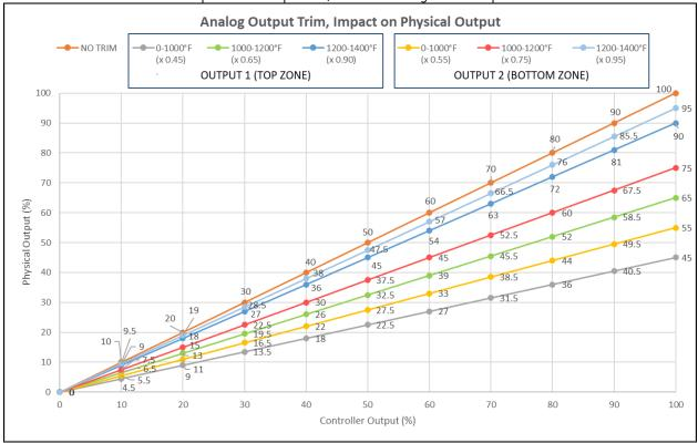
As an example, if the controller requires 60% Output to maintain 1300°F, the Top Zone will receive 39% Output (or 10.24 mA), while the Bottom Zone will receive 45% Output (or 11.2 mA). This small difference may improve the Temperature Uniformity within the furnace.
