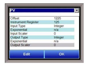
The Process Variable (PV), Setpoint (SP), and Output (Out) can be set up from this screen. Select the desired option from the drop-down list to configure those settings.
