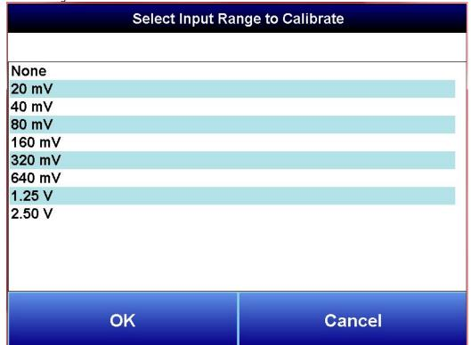
3. Check the inputs that will be receiving the signal (the inputs will be filtered based on the input range selected in step two so that only relevant inputs can be calibrated).
