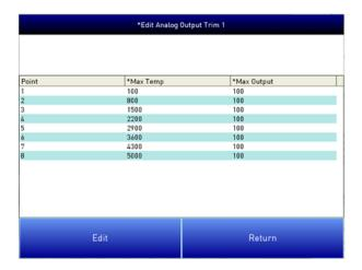
The Analog Output Trim <u>must</u> be assigned to a Physical Analog Output (see **Analog Output Setup -> Output # -> Assignment**, and select **Trimmed Output #, Loop #**). When assigned to an Analog Output, the physical output will represent:
