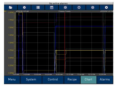
The folder button - allows you to load files to view.
