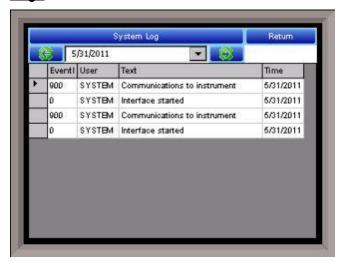
The Logs screen will allow the user to view three different types of logs – **System, Alarms,** and **Cycle**.
