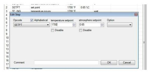
Under the Atmosphere Setpoint text in the upper middle portion of the Edit Step box, there is a numeric entry box. To modify this setpoint, either the Up or Down arrows can be pressed, or the desired atmosphere level can be entered into the box from a keyboard. Once the correct setpoint has been entered, press the OK button in the bottom right corner of the Edit Step box.
