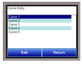
Most types of inputs that are used in SSi controllers are already setup with a curve built for most every type of thermocouple available, certain vacuum sensors, etc. However, if an application calls for an input without a standard curve, the curve can be built using this option. Voltages can be paired with corresponding values to create a sensor curve based off of a provided equation or data. This allows the controller to make appropriate readings from the sensor.
