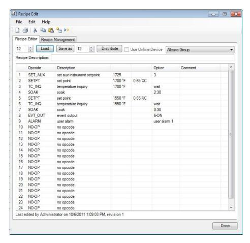
Before adjusting the recipe, the operator must first understand what needs to be modified. For example, if the atmosphere level needs to be adjusted at the beginning of the recipe, double click on the line for SETPT. The SETPT Edit Step box will appear.
