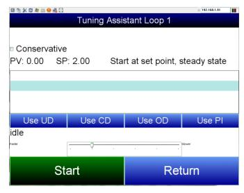
The "Conservative" option will allow the user to minimize, if not remove, the possibility for an overshoot of the setpoint. If a small overshoot is acceptable, leave the "Conservative" checkbox unchecked. If, however, no overshoot is desired, then checking the "Conservative" checkbox will accomplish this.
