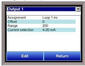
The NitroMeth Plus Controller has the option of six analog outputs. The outputs are ranged for a 4-20 milliamp signal or a 0-20 milliamp signal. Each output comes with a factory default configuration dependent on the application. Each output can be modified prior to shipment to your facility or in the field by a supervisor.
