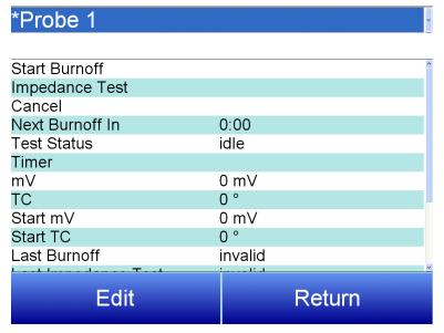
The Burnoff menu manages various burnoff settings and functions. Use the drop down menu at the top of the screen to select the desired Probe.
