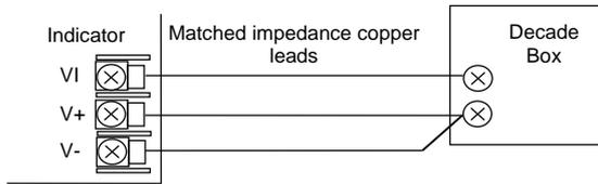
The RTD range of the instrument is -200 to 850°C. It is, however, unlikely that it will be necessary to check the instrument over this full range.
