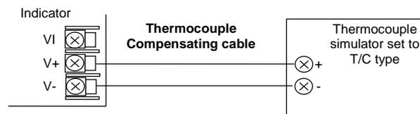
Set the mV source to the same thermocouple type as that configured in the indicator.
