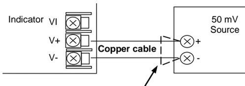
For best results 0mV should be calibrated by disconnecting the copper wires from the mV source and short circuiting the input to the indicator
