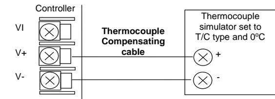
Set the mV source to **internal compensation** for the thermocouple in use and set the output for **0mV**. Then:-
