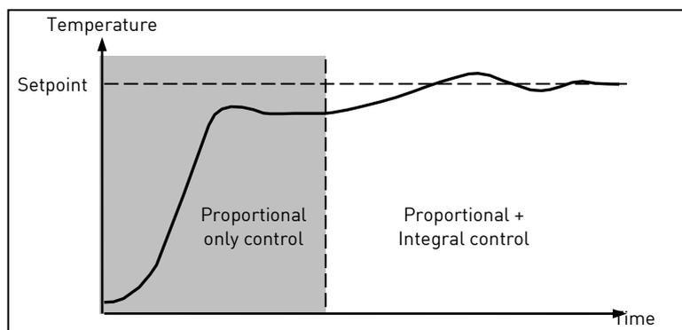
The units for the integral term are measured in time (1 to 9999 seconds). The longer the integral time constant, the more slowly the output is shifted and results in a sluggish response. Too small an integral time will cause the process to overshoot and even oscillate. The integral action may be disabled by setting its value to OFF.
