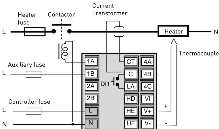
**Note:** a burden resistor value 10Ω is mounted inside the controller.
