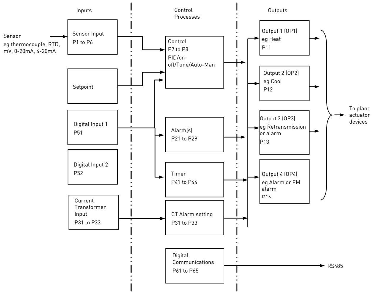
The Temperature (or Process Value, PV) is measured by the sensor and compared with a Setpoint (SP) set by the user.
