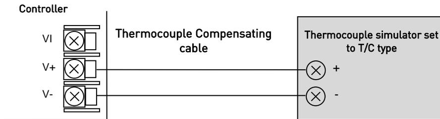
Set the mV source to the same thermocouple type as that configured in the controller.
