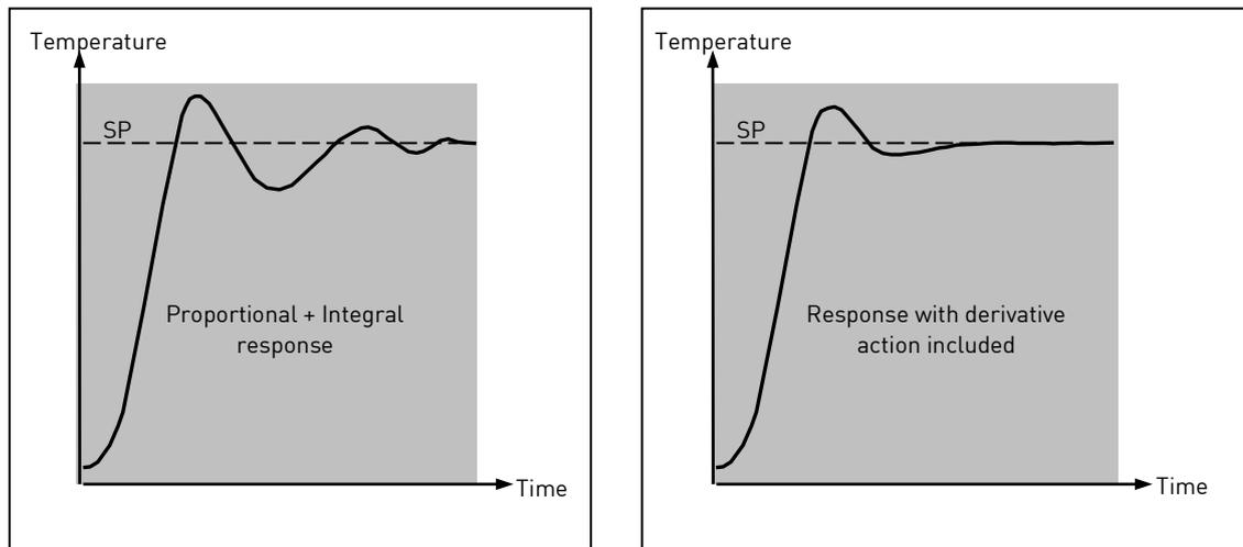
The derivative modifies the output to reduce the rate of change of error. It reacts to changes in the PV by changing the output to remove the transient. Increasing the derivative time will reduce the settling time of the loop after a transient change.
