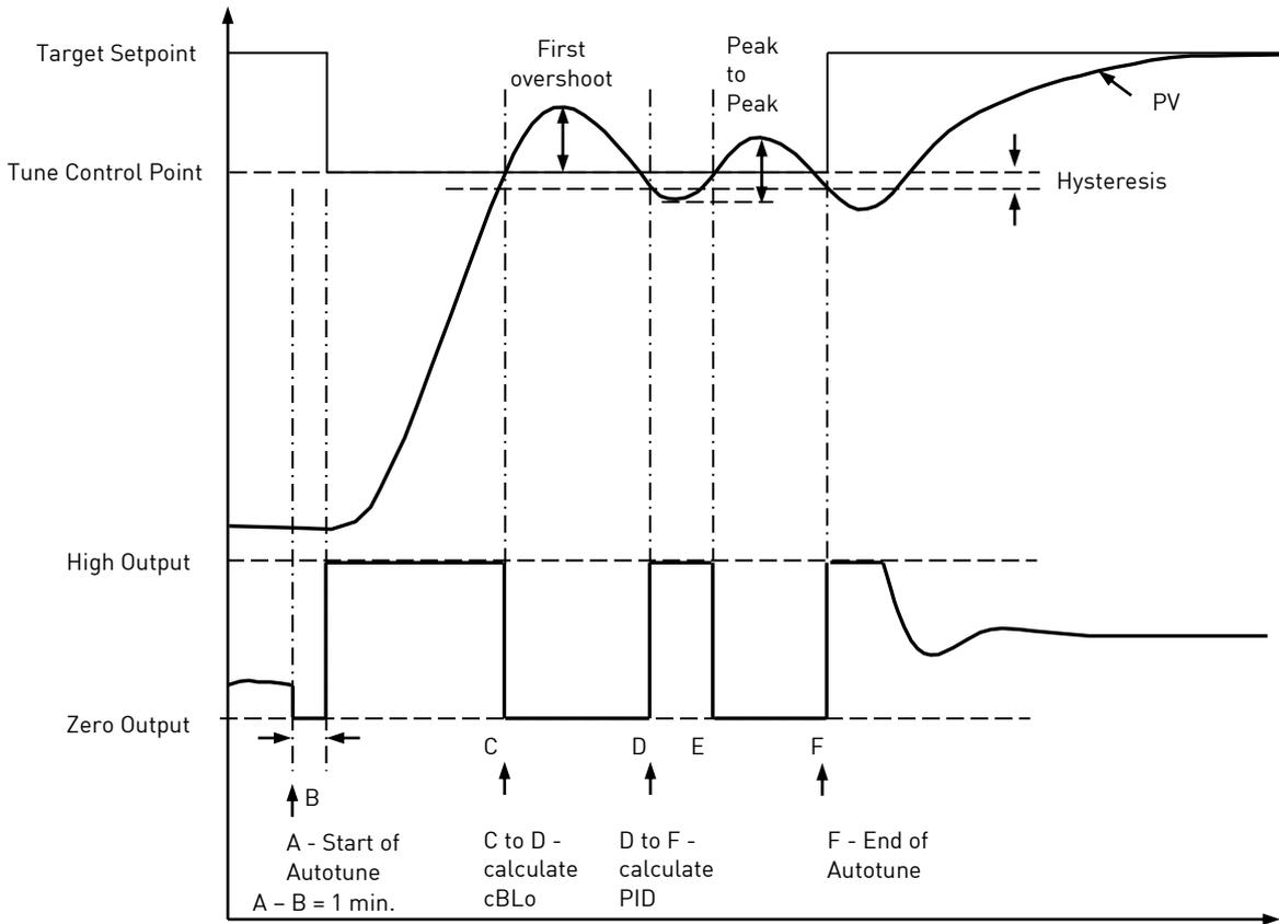
For a tune from below setpoint 'cBL0' is calculated on the basis of the size of the overshoot (assuming it was not set to Auto in the initial conditions). 'cbHi' is then set to the same value as 'cBL0'.
