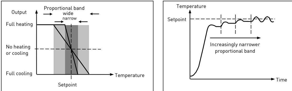
The diagram also shows the effect of narrowing proportional band to the point of oscillation. A very wide proportional band results in straight line control but with an appreciable initial error between setpoint and actual temperature. As the band is narrowed the temperature gets closer to setpoint. If the proportional band is very narrow the loop becomes unstable resulting in an oscillatory response.
