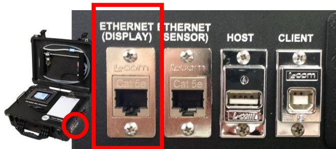
Figure 12 - Location of Ethernet port for cable connection
