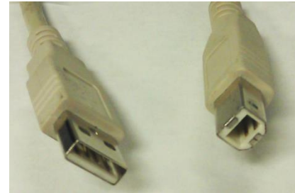
Figure 7 - USB connection types Standard-A (left), Standard-B (right)
