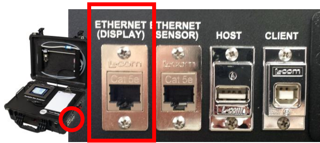
Figure 10 - Location of Ethernet port for cable connection
